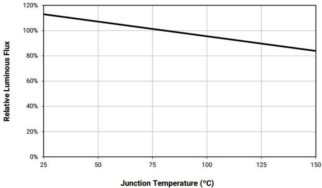
**Figure 3: Relative flux depreciation of the XLamp XB-D with increasing junction temperature<sup>9</sup>**
