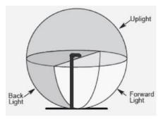
Figure 4: Backlight and uplight emitted by a typical HID outdoor light<sup>10</sup>
