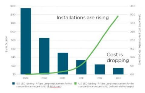
Figure 2: Average cost of LEDs per 1000 lumens and estimated number of LEDs installed in the U.S. (sourced from the U.S. Office of Energy Efficiency and Renewable Energy<sup>8</sup>)
